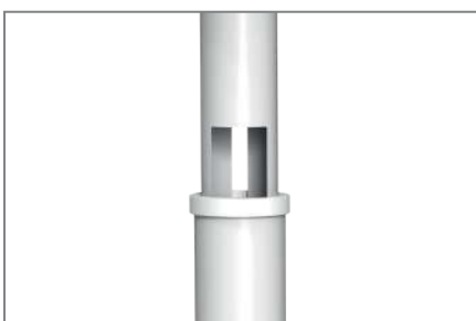
cable management within the telescopic tube
