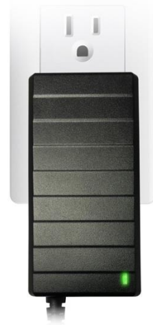
Green indicates charging complete
