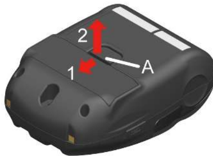
Figure 15-1 Removing Battery Pack (1)
