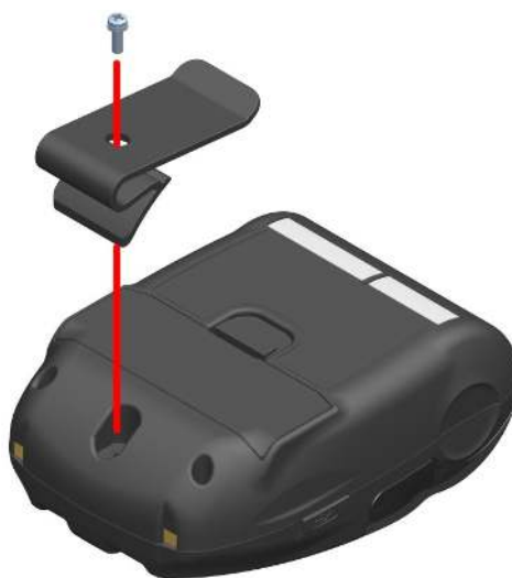
Figure 13-1 Attaching/Detaching Belt Clip
