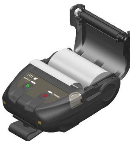
Figure 9-3 Thermal Paper Setting Direction Example
