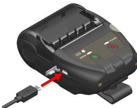
Figure 8-1 Printer and USB Cable Connection
